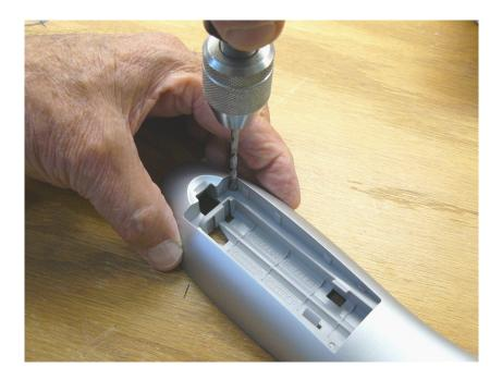
to make a hole at the right rear corner of the battery compartment, as shown in the picture above. Hold the bit against the corner as you drill, so that the hole is as close to the corner as possible. Remove burrs or sharp edges around the hole with a knife, a small file, or whatever.
