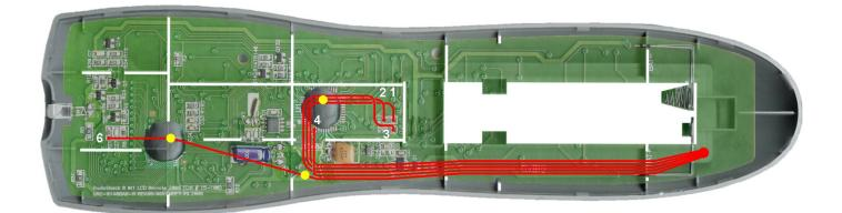
In the picture above, you are looking down at the circuit board through a ghost image of the lower case, so you can see roughly how the cable will be routed. The white areas show the footprint of the ribs which support the circuit board, and you must route the cable so it clears them. The yellow dots are recommended points to anchor the cable to the board with hot glue. They're not absolutely necessary, but help to keep the cable from shifting and straining the solder joints.
