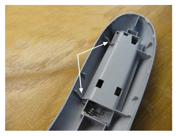
Cut "V" shaped notches in the two ribs on the cable side of the lower case, as shown in the picture above.
