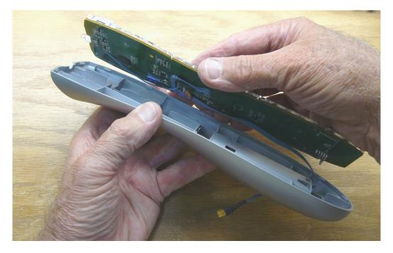
side ribs, and that no part of the cable is pinched between the board and the lower case. If the board doesn't feel firm against the case, it is probably because one or more wires are caught between the board and one of the ribs. Work on this until you are convinced the board is resting solidly on all portions of the ribs that are level with the surface of the battery compartment.
