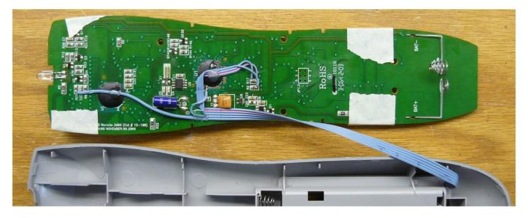
Lay the circuit board beside the lower case, and give the cable a half twist so it looks like the above picture. Start by soldering wire #6 to the bottom end of R21. If there is not a generous amount of solder on the resistor already, add some. Pass wire #4 either over or under the group of three, lay the end in the space between the two fingers you previously tinned, and solder it to both of them, as shown below.
