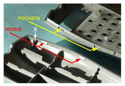
Each snap-latch consists of a hook on the upper inside edge of the lower case, and a corresponding pocket in the lower outside edge of the upper case, as shown above. The general procedure is to pry open these latches one at a time with a thin blade, using shims to hold them open until the case can be separated. Easier said than done. For example, ribs in the lower case (such as "X" above) can interfere with inserting or sliding the blade.
