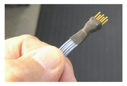
The final step is to place the end of the heat shrink over the edge of a table while it is still hot and soft, and press down with something smooth to flatten it tightly against the ribbon cable. If you do a really nice job it may look as good as mine, shown above. This is a good time to mark the corner where pin #1 is located, using a spot of fingernail polish.
