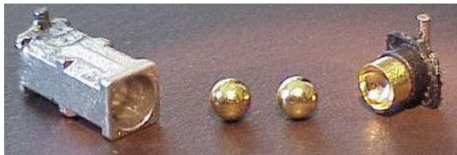
Figure 4. Disassembled Motion Sensor Switch
